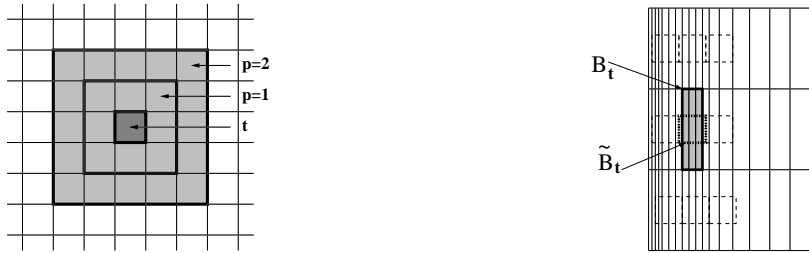
FIG. 5.2. Left: The first two layers p = 1 and p = 2 around the box \tilde{\mathcal{B}}_t of t . The first layer consists of 9 boxes, the second one of 25 boxes (it includes the first). Right: A cluster t with box \tilde{\mathcal{B}}_t that is much smaller than the bounding box \mathcal{B}_t of \Gamma_t . The dashed boxes \tilde{\mathcal{B}}_s correspond to non-empty clusters s .
